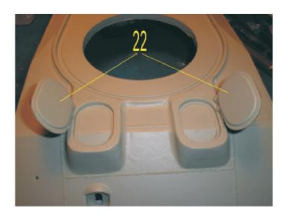
Install lift ring on right as shown.
