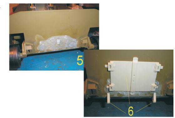
Use 1mm copper wire or paperclip and form a handle as shown. Use CA glue to attach or carefully use a soldering gun to heat the copper till it melts into the doors.
