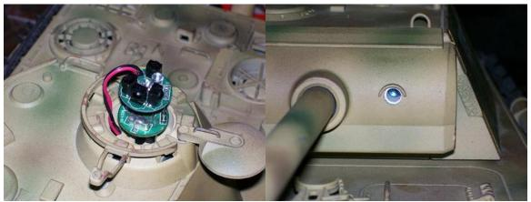
Yes. See the following pics on how I mounted my IR emitter in my Panther's mantlet. I mounted the emitter in a plastic tube with the tip of the emitter recessed 9mm from the opening of the tube. This gives the IR beam a tight pattern vs a shot gun light spray. The 9mm recess is widely recognized as the IR battling standard, but check with your local club first.
