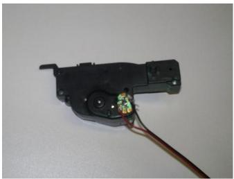
It has been discovered that the polarity of the Heng Long recoil/airsoft motor is opposite of the wire (red + / black -) that comes with the SLU kit. You will want to reverse the connections as to not damage the recoil/airsoft motor. So wire the red from the SLU to the negative on the motor, black from the SLU to the positive on the motor. The above pic has the correct wiring.
